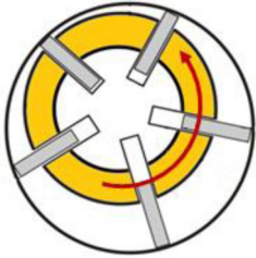
Figure 23. Schematic of thin film contributing to viscous friction between rotor sides and housing.
