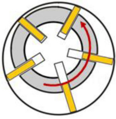
Figure 24. Schematic of thin film contributing to viscous friction between vane sides and housing.
