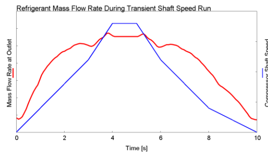
Figure 13: Compressor refrigerant mass flow rate predictions under transient speed ramp operation.
